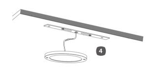
4 Pull the power cord through the frame and connect the wires.
